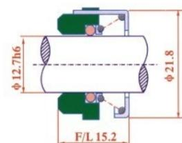
For Mats NL/SA, Mits FX105V, Sanden(三电)SD505/575/507Mini, Sanden(三电)SDTR70/90/105, Compressor
