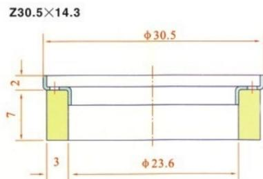
For Sanden(三电)sd507/508/510 felt wiper ring with retainer
