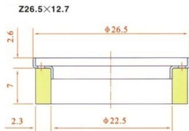
For Sanden(三电)sd505/507 mini felt wiper ring with retainer
