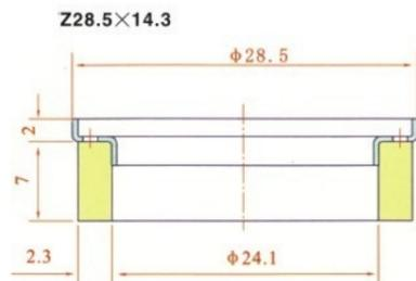
For Sanden(三电)sd708/709/two piece felt wiper ring with retainer
